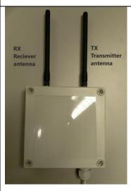
Make sure to tighten the cable gland so that it firmly holds the cable
